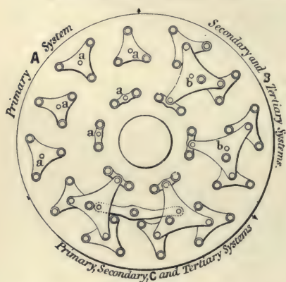
FIG. 75.—Primary, secondary, and tertiary systems of levers shown separately.
